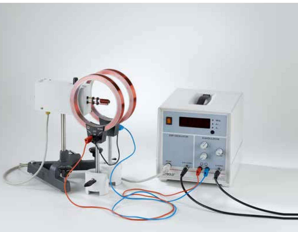
Electron spin resonance on DPPH (C3.4.4.1)
